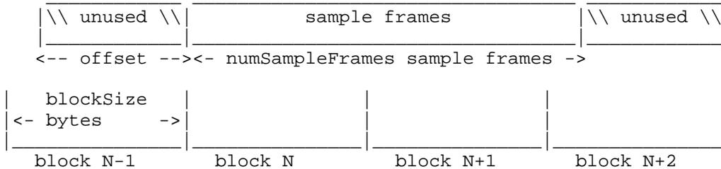
Figure 5-Block-Aligned Sound Data
